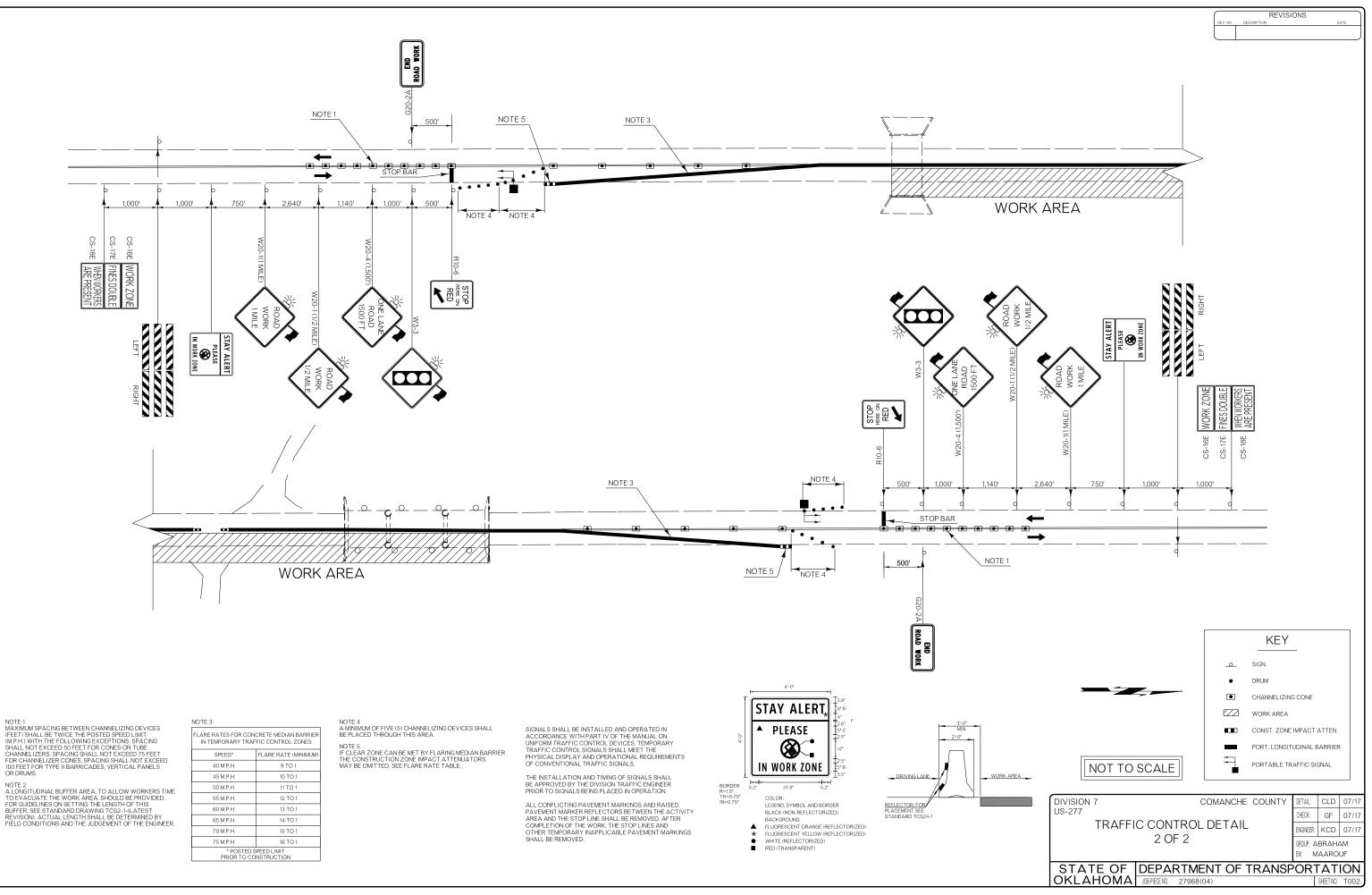
NOTE 1 MAXIMUM SPACING BETWEEN CHANNELIZING DEVICES (FEET) SHALL BE TWICE THE POSTED SPEED LIMIT (M.P.H.) WITH THE FOLLOWING EXCEPTIONS. SPACING SHALL NOT EXCEED 50 FEET FOR CONES OR TUBE CHANNELIZERS. SPACING SHALL NOT EXCEED 75 FEET FOR CHANNELIZER CONES, SPACING SHALL NOT EXCEED 100 FEET FOR TYPE II BARRICADES, VERTICAL PANELS OR DRUMS.
